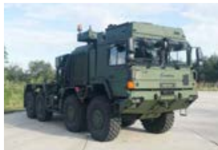
HX2 – 45M, Multiple towing concepts combined with the highest available lift capacity leave no vehicle unrecoverable.
